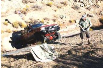
Rigging a "floating" pulley. 2nd parachute will be added next.
